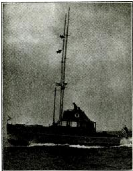
Fig. 2. Corsair II , a sport fishing cruiser owned by Lt. Everett Walsh of the South Shore (L. I., N. Y.) Power Squadron is a typical installation in which the tall outrigger poles support aerial wires (arrows) which run their entire length down to the deck below.
